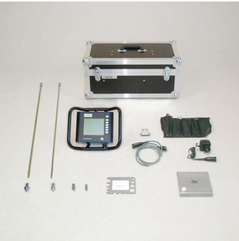
Figure 10b. Proposed penetrometer to assess soil penetration resistance. Use same devise for all sites: Eijkelkamp, Giesbeek, The Netherlands
