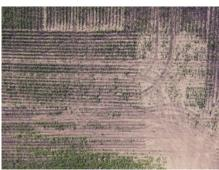
**Compaction** is the destruction of natural aggregates and rearrangement of soil particles to form more or less continuous masses of hard, high bulk density soil. Compaction occurs when a direct load is applied that exceeds the soil's bearing capacity and is caused by tractor and machinery traffic, tillage and intensive grazing. Compaction must be prevented because it is very difficult to reverse.
